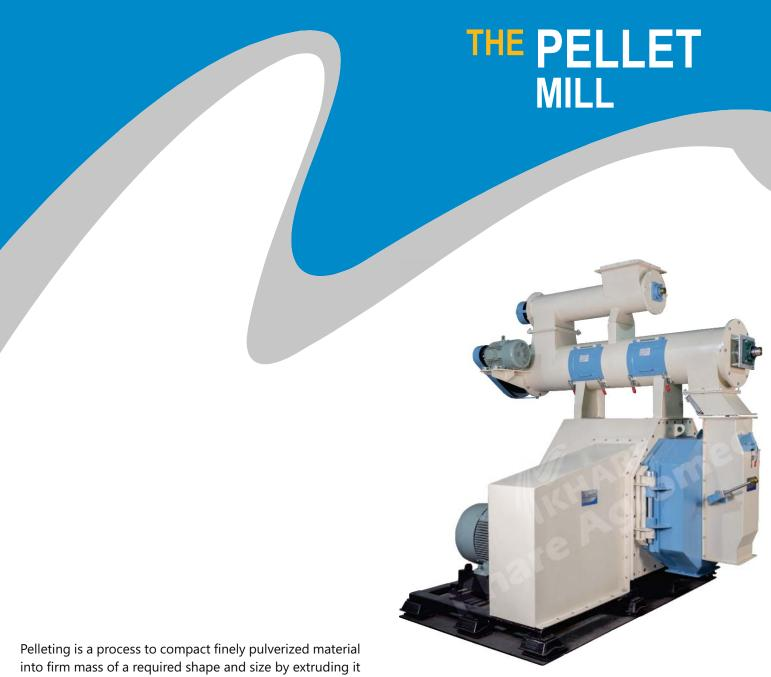
Pelleting is a process to compact finely pulverized material into firm mass of a required shape and size by extruding it through a metalic ring die. Finely ground material is fed into the Pellet Mill through a feeder and then pressed into a rotating ring die with the help of two press rolls free to rotate on their respective shafts. The resulting pressure compresses the material and extrudes it through the holes in the die
